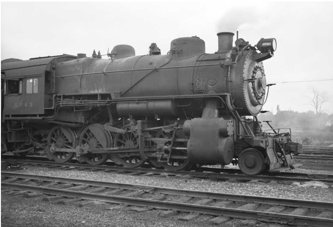
A second look at a PRR class H-10, 2-8-0 locomotive at Sandusky. A close up of No. 9943 for the modelers. Photo by Donald A. Kaiser, 1955-56.
